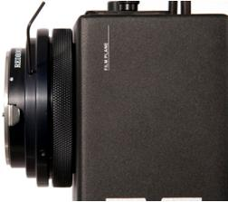
The set closest to the lens is used to change lens mounts. Unscrew all three of them, and remove the lens mount. Replace the current lens mount with the new one.
