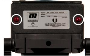
Unscrew both sets of screws and place two AA rechargeable batteries. We currently ship the Encore with AA NiMH 2000mAh batteries, though other mAh ratings will work.
