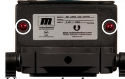
Unscrew both sets of screws and place the two AA rechargeable batteries that are included in the box.
