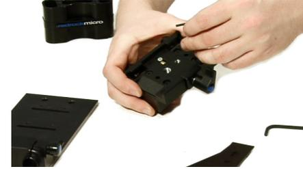
4) Finally, screw the low riser back onto the cheeseplate using the original four screws.
