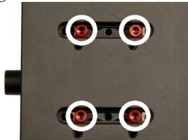
2) Next remove the quick release sliding plate from the base to reveal two more sets of screws. Unscrew all four screws.
