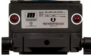
Unscrew both sets of screws and place the two AA rechargeable batteries that are included in the box.
