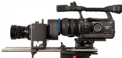
Your M2e unit should line up with the camera, and the lip of your achromat should slip into the blue coupler attached to the MicroX. Tighten down the three tension screws to complete assembly.
