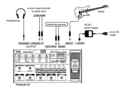
Use audio cables to connect ToneLab LE's OUTPUT L/MONO and R jacks (7.6) to a mixer/ recorder or guitar amp. If desired, you can also connect an external effect processor. To do this simply connect SEND to the input of your external processor, and RETURN to the output of your external processor.
