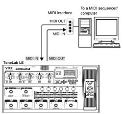
When you connect ToneLab LE with a MIDI sequencer or sound editor, data will normally be sent in both directions, so you will need to connect MIDI cables from ToneLab LE's MIDI OUT jack to the external MIDI device's MIDI IN jack, and from the external MIDI device's MIDI OUT jack to ToneLab LE's MIDI IN jack.
