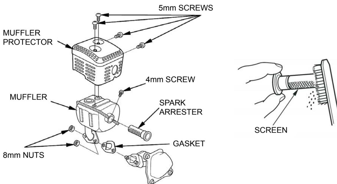
4. Use a brush to remove carbon deposits from the spark arrester screen. Be careful to avoid damaging the screen.
