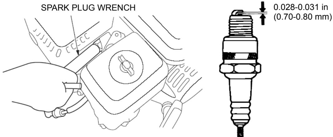
3. Inspect the spark plug. Replace it if the electrodes are worn, or if the insulator is cracked or chipped.
