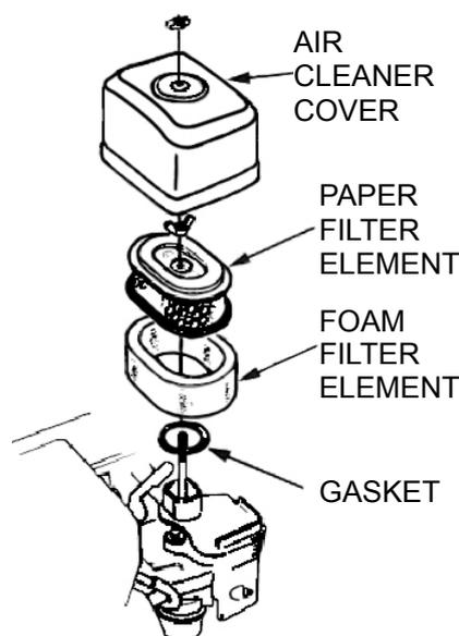
Paper air filter element: Tap the filter element several times on a hard surface to remove dirt, or blow compressed air [not exceeding 30 psi (207 kPa)] through the filter element from the inside. Never try to brush off dirt; brushing will force dirt into the fibers.
