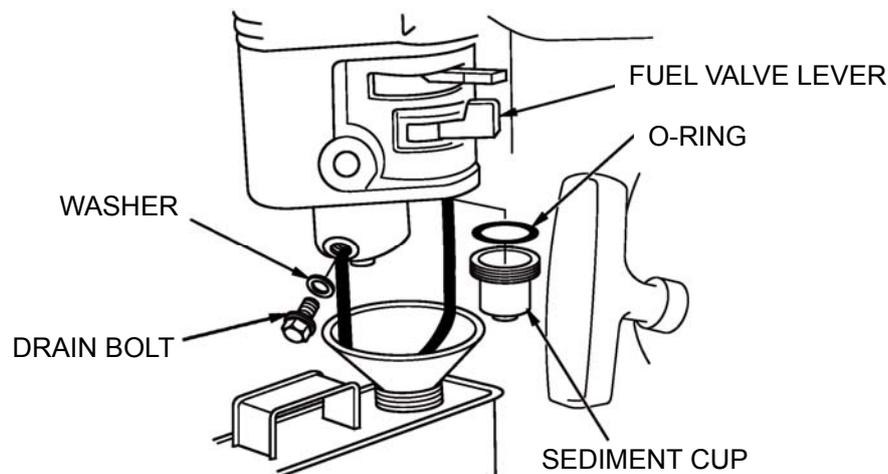
3. After all the fuel has drain into the container, reinstall the drain bolt and sediment cup. Tighten them securely.
