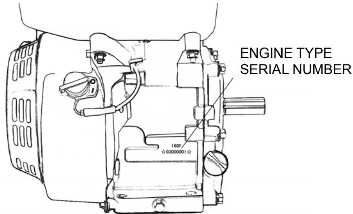
Record the engine serial number in the space below. You will need this serial number when ordering parts, and when making technical or warranty inquiries.
