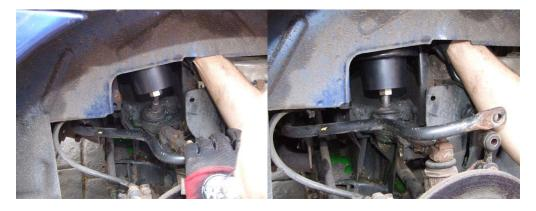
23. Follow the same set up process as described in step 13, noting that the rear springs are higher rated and so the pre-tensioning does make this much stiffer to turn.
