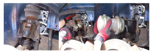
11. Retain the spacer washer that sits over the shaft of the 'knuckle' and clean off any dirt or corrosion. The spring found between the 'Knuckle' and displacer is not refitted. A light smear of copper grease will help reduce any future sticking problems. Check the rubber bump stop is in place and not been damaged or lost. If lost or damaged then a replacement will be needed.
