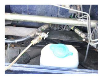
4. The right side suspension needs to be depressurised (not the left side at this time) and the image shows the use of a correct Hydrolastic pump with the correct adapter that screws onto the valve and the pressure is contained within the pump. Moving the control lever from 'pressurise' to 'depressurise' allows simple and safe depressurisation of the suspension and the collection of the fluid inside the pump reservoir.
