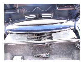
18. To access the rear right top damper mounting and the displacers fluid connection requires the coolant expansion tank to be moved. It is held in place by two 8mm headed bolts and an extension 'peg' on the tanks moulding underneath. With the bolt removed the tank can be lifted up and the lower 'peg' disconnects. Stretch within the hoses does allow it to be moved to the side and above the dipstick and oil filler.
