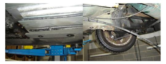
The pipes should remove freely from underneath the car.
