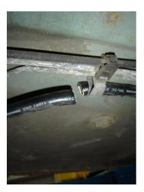
Once cut lower the pipes which were connected at the front and gentle pull the Hydragas pipe through
