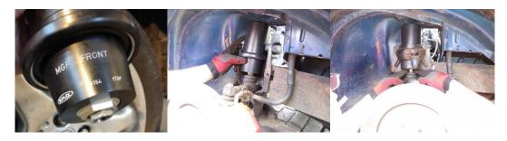
13. Once fitted in place, Using a felt pen or similar mark the front flat of the hexagon, wind out the hexagon adjuster from the SUPLEX suspension unit by 18 turns. Fit the locking ring to the threaded adjuster but do not tighten.
