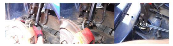
16. Refit the horns and electrical connections and then refit the plastic under wing shields.
