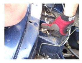
9. Place a fluid catch tray under the displacer position to collect spilt Hydrolastic fluid, and leave it there until you have finished this side. From inside the under bonnet area loosen the nut clamping the Hydragas pipe to the displacer. Remove the pipe from the displacer and push it downwards to allow some fluid to drain into the tray. Leave it there until you have also removed the rear displacer connection as further fluid will drain when the rear is disconnected.
