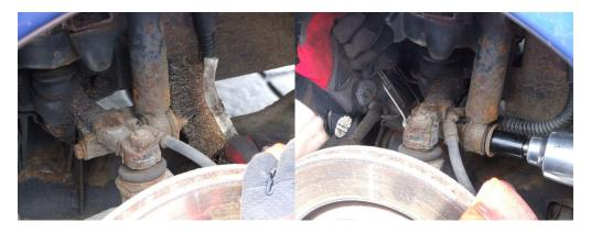
8. The damper is now hanging from the top fixing only, and best access to this is achieved by unclipping the electrical plug connections to the horns and then removing them and their brackets from the cars chassis leg.
