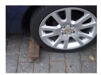
The next action is to loosen the wheel nuts on that side and raise the right side of the car to a
