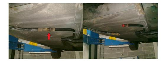
Once disconnected from these points the pipes which runs along the chassis from front to rear can be capped using the red blanking caps (supplied in the kit).
