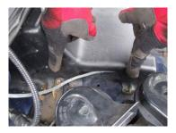
• On the left side of the car is a scrivet holding the moulding to the heater air intake vent. (A scrivet is a two piece combination of a plastic screw and plastic rivet, where the screw centre pushes out 'wings' of the outer rivet when it is inserted.) Unscrew the central screw using a cross head screwdriver and then prize out the rivet section.
