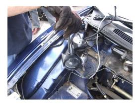
Damper removal will require the top shaft of the damper being held whilst the nut is loosened with a spanner. Once the nut is loose take hold of the damper body with your now spare hand to prevent the damper dropping out when the nut is spun off. Remove the upper washers and rubber bush.
