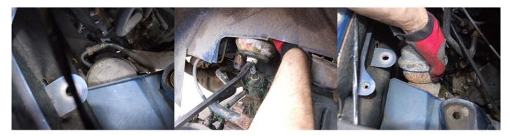
22. Select a SUPLEX rear suspension unit and fit this in from the wheel arch and 'post' it up between the body and subframe, before negotiating it into position is the same way as described in step 12.
