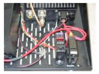
The keying wiring connects the keyer and front panel key jack to the radio, and the radio to the amplifier.
