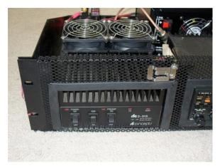
cover, and position it in place on the rack shelf. Observe where components are located in the amplifier, and then drill four holes through the shelf slots and up into the amplifier case. Alternatively, L-brackets that secure to the screws on the side of the case to the heatsink could be used.
