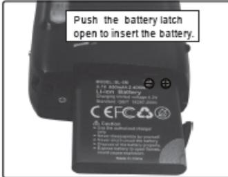
Make sure the battery has been inserted properly into your digital camera, according to the polarity shown inside the battery compartment.
