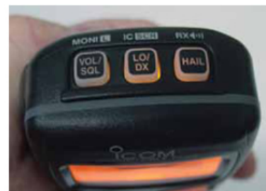
Testers found the CommandMic III's flush-mounted top buttons hard to use one-handed.
