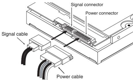
**Figure 10. Attaching SATA cabling**
