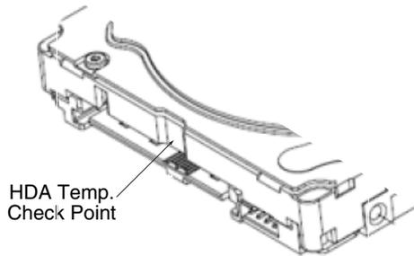
Figure 9. Location of the HDA temperature check point
