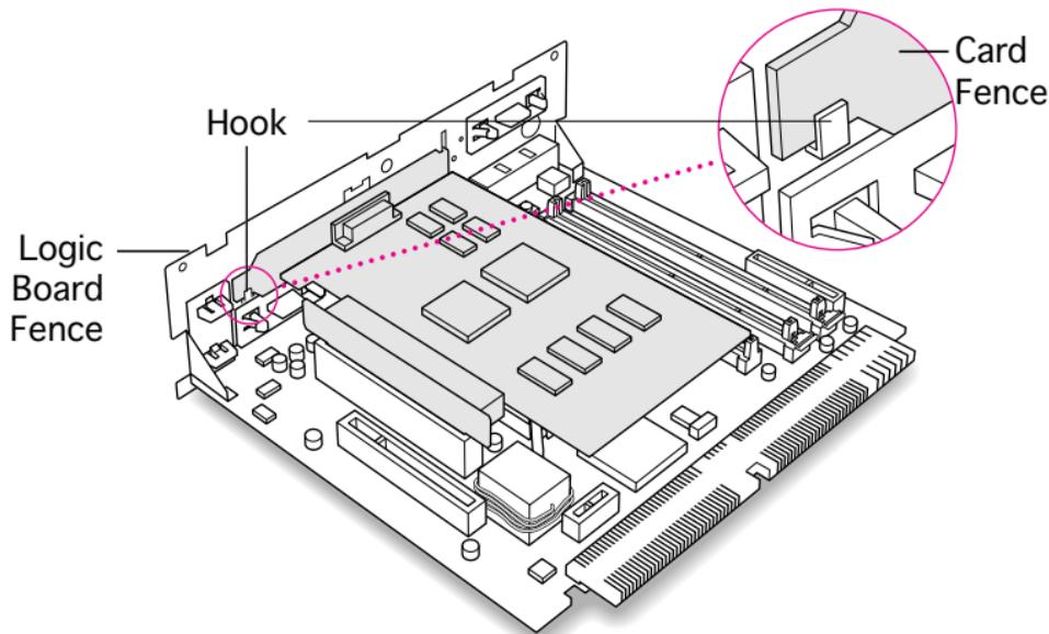
10 Be sure the PCI connector is in the access port and accessible outside the logic board fence.
