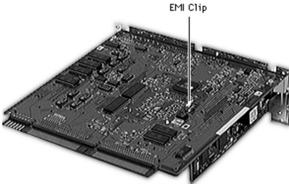
**Caution:** Take care to avoid compressing the EMI clip on the bottom of the logic board. If possible, support the underside of the board to avoid compressing the silver-colored EMI clip.
