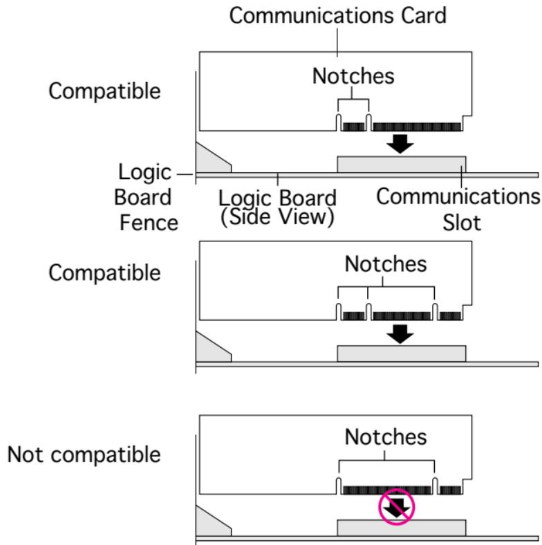
**Note:** Some communications cards are not compatible with this computer. Examine the placement of the notches on the card. Use these illustrations as a guide to identify the correct type of card for the slot.
