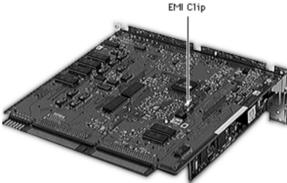
**Caution:** Take care to avoid compressing the EMI clip on the bottom of the logic board. If possible, support the underside of the board to avoid compressing the EMI clip.
