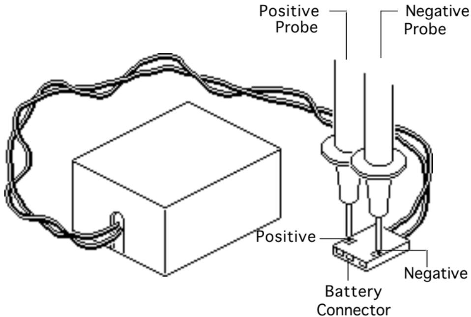
Set the voltmeter to the 10 VDC scale.
