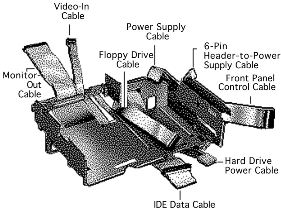
**Replacement Note:** Arrange the cables as shown before replacing the shield/wiring harness. When dressing the cables, do not crimp them between the harness and the floor of the bottom case, or between the harness and the sides of the bottom case. Route the speaker cable between the logic board connector and the CD-ROM shelf. Route front panel control, power supply, and header cables to the side of the front panel control bay.
