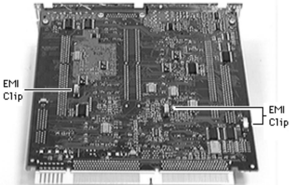
**Caution:** Take care to avoid compressing the EMI clips on the bottom of the logic board. If possible, support the underside of the board to avoid compressing the three silver-colored EMI clips. (The Performa 6360/160 has only one EMI clip.)
