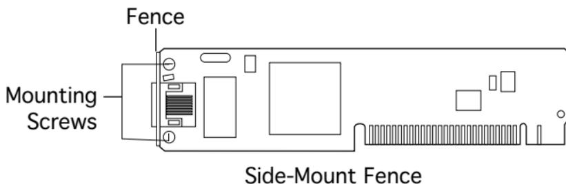
**Replacement Note:** If you are installing an Ethernet card and its fence does not include a hook, replace the fence.
