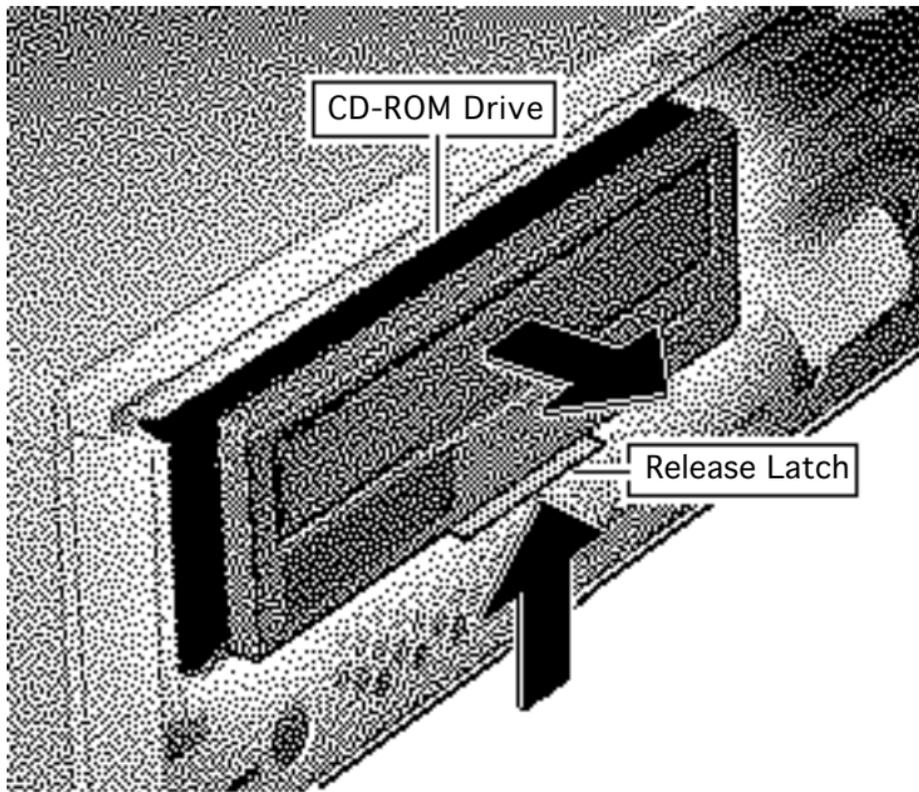
**Note:** To perform the next procedure, you may want to insert a flat-blade screwdriver in the slot of the release latch to help you pull out the CD-ROM drive.
