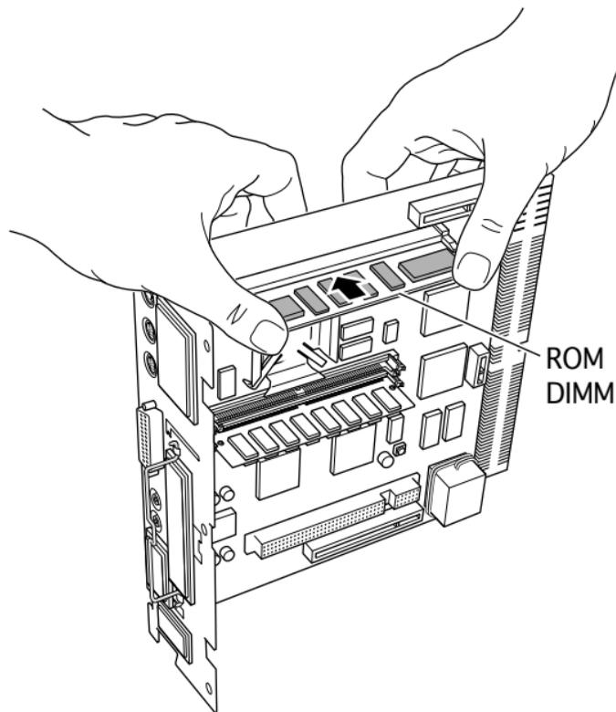
10 Hold the logic board vertically with the communications slot end of the board resting on your workspace.
