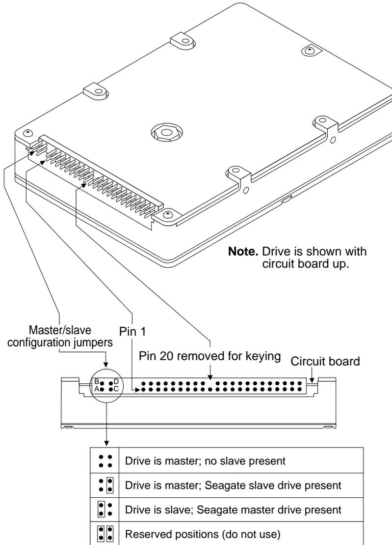
**Figure 11. ST9235A and ST9235AG connector setup**
