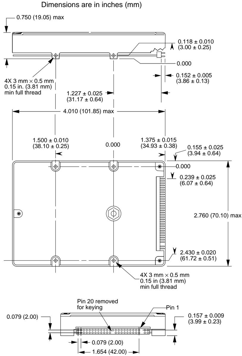
**Figure 7. ST9235A and ST9235AG mounting dimensions (MCC mounting version)**
