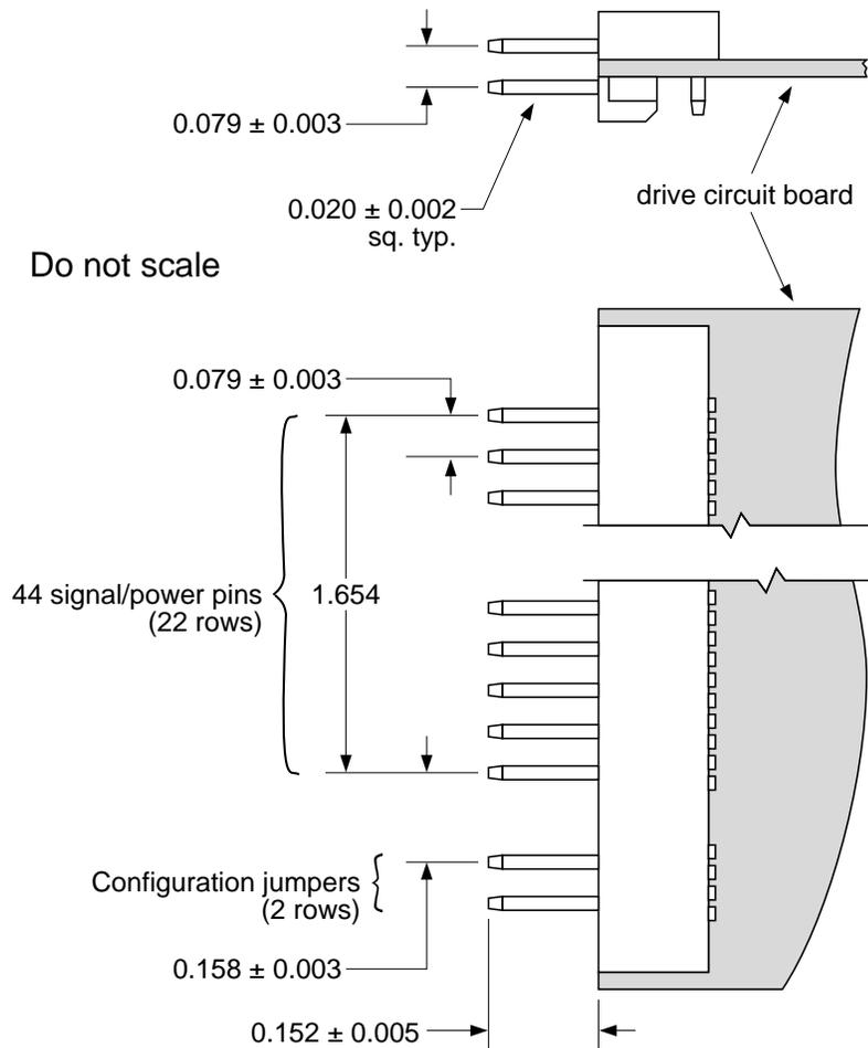
Figure 12. ATA interface connector diagram
