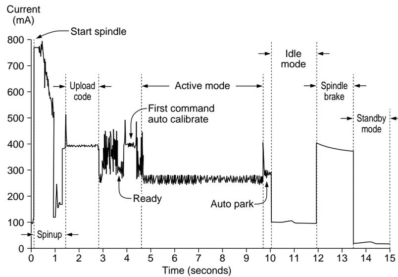
**Figure 1. Typical startup and operation current profile for the ST9080A**
