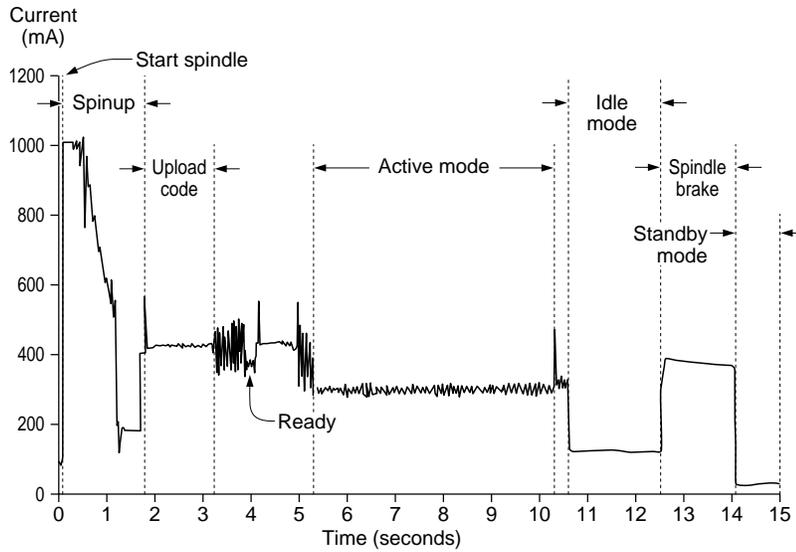
**Figure 3. Typical startup and operation current profile for the ST9235A and the ST9235AG**
