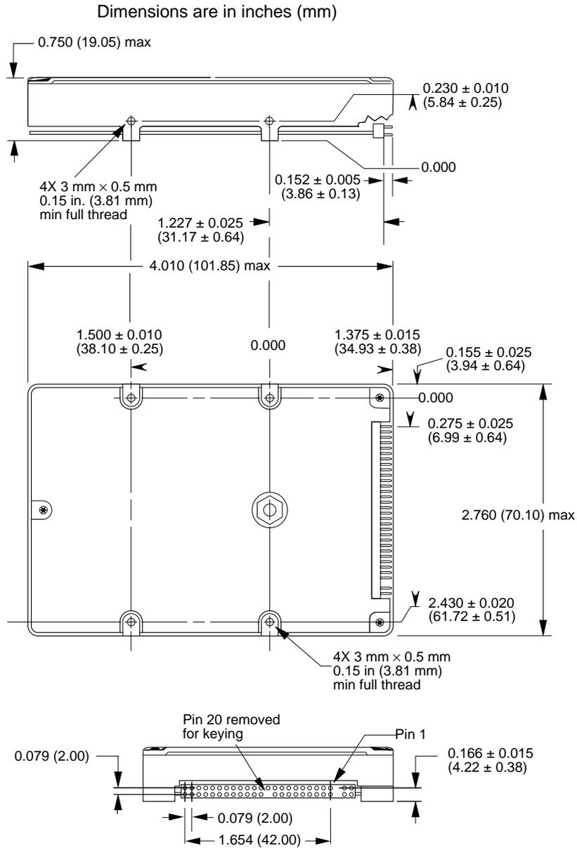
**Figure 8. ST9235A and ST9235AG mounting dimensions (non-MCC mounting version)**
