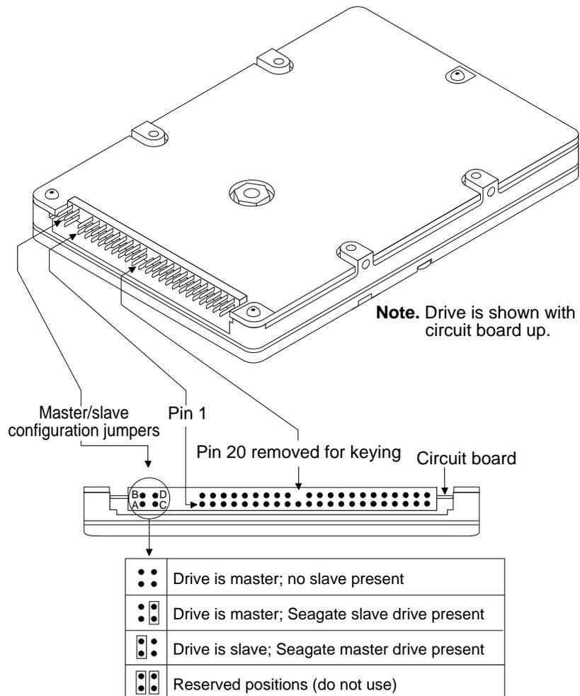
**Figure 9. ST9080A connector setup**
