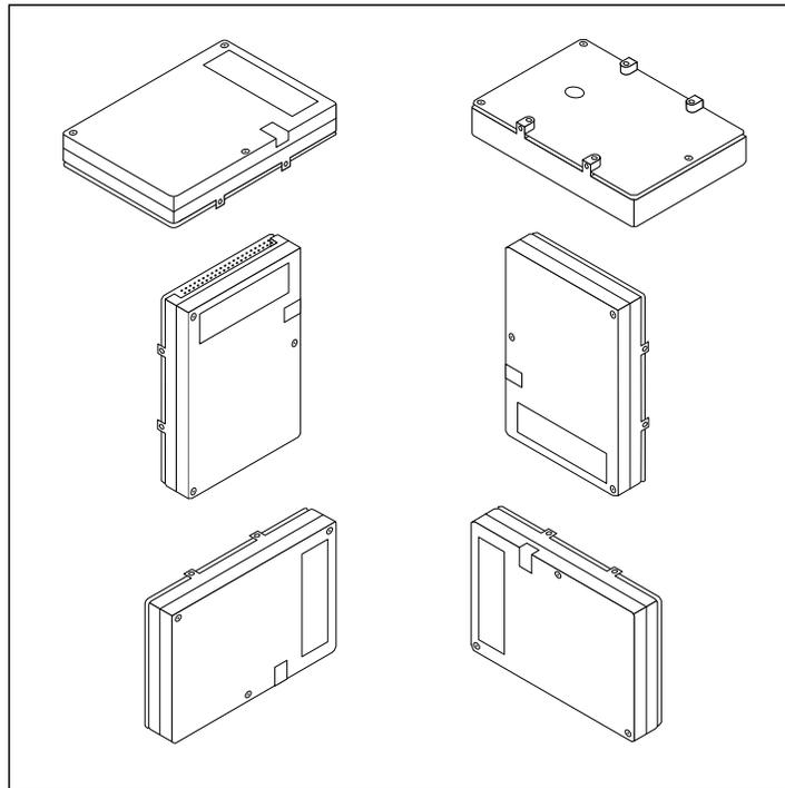
Figure 4. Acceptable mounting orientations for the ST9235 family drives
