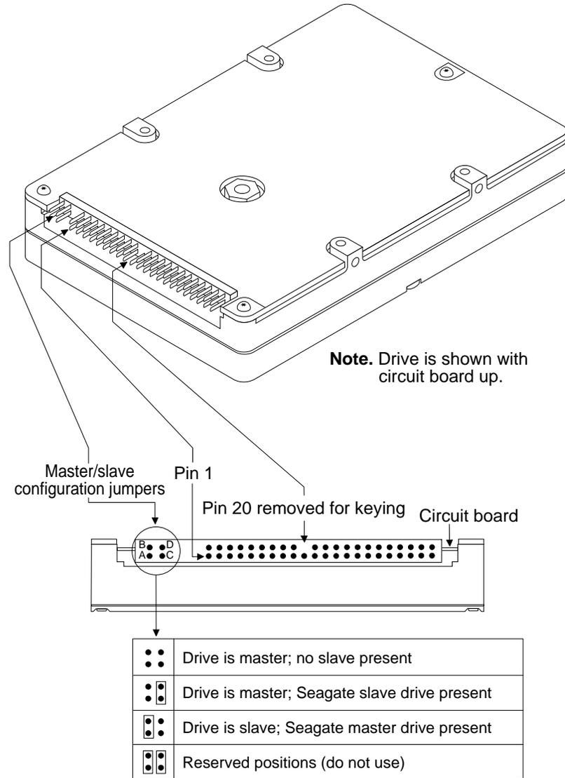
**Figure 10. ST9145A and ST9145AG connector setup**
