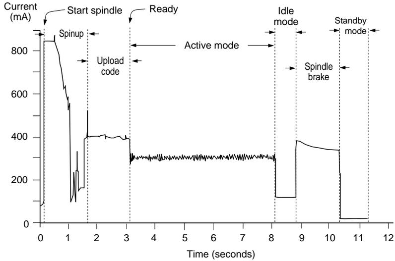
**Figure 2. Typical startup and operation current profile for the ST9145A and the ST9145AG**
