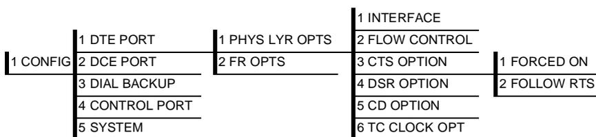
**Figure 3-2. Example of Basic Front Panel Menu Navigation**
