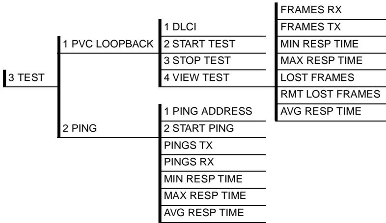
**Figure 11-2. Front Panel Test Menu**
