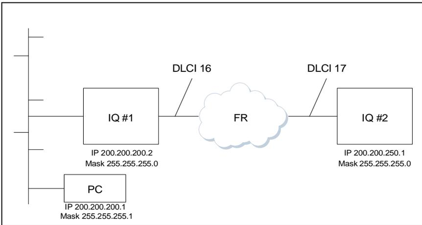
**Figure 3-5. PC Connected to Local and Remote IQs**
