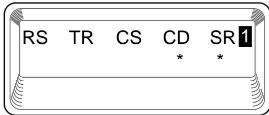
**Figure 10-12. Control Signal Status Screen**
