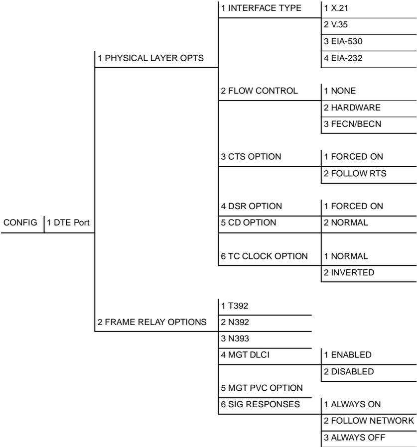
**Figure 5-2. Configuration Menu Tree for DTE Port**
