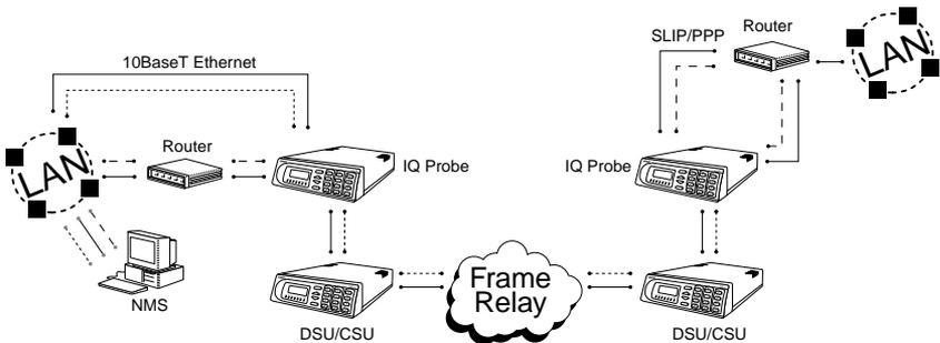
**Figure 4-2. Out-of-Band Management Application Example**
