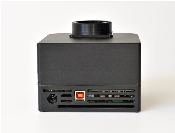
Illustration 10: Power connector (left) and USB connector (right) on the bottom side of the camera head
