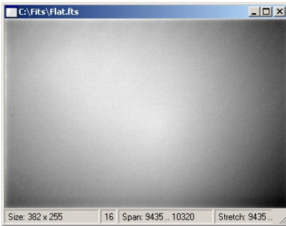
Illustration 20: Flat field represents the telescope/camera response to uniformly illuminated field
