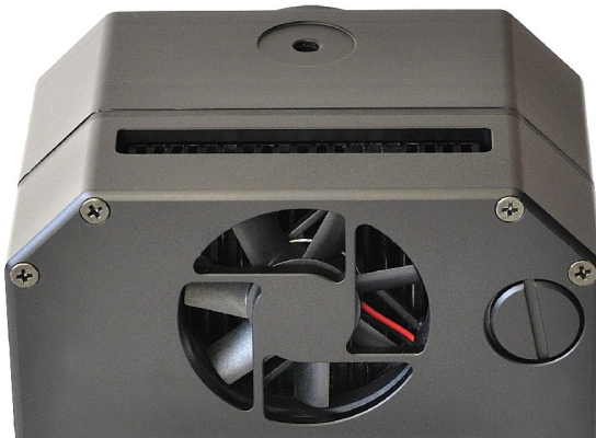
Illustration 26: Silica-gel container is under the screwed cap with slot, right of the fan vents
