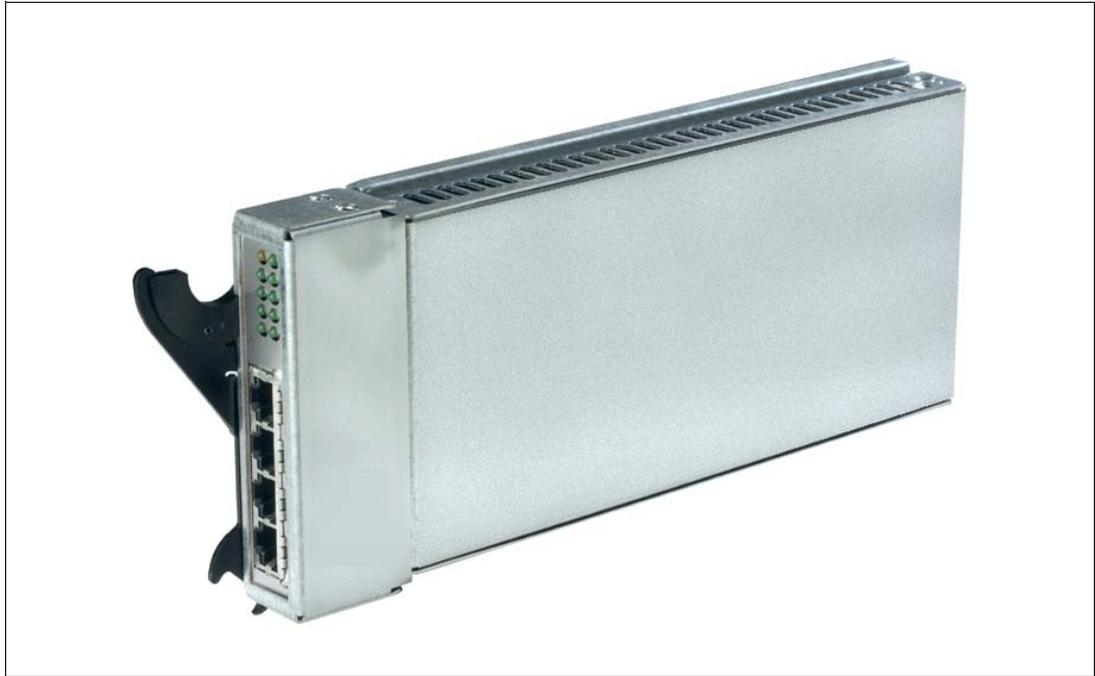
Figure 1-10 BladeCenter 4-Port Ethernet Switch Module
