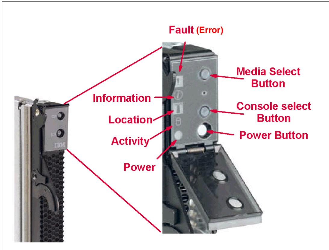
Figure 1-5 Blade server operators panel
