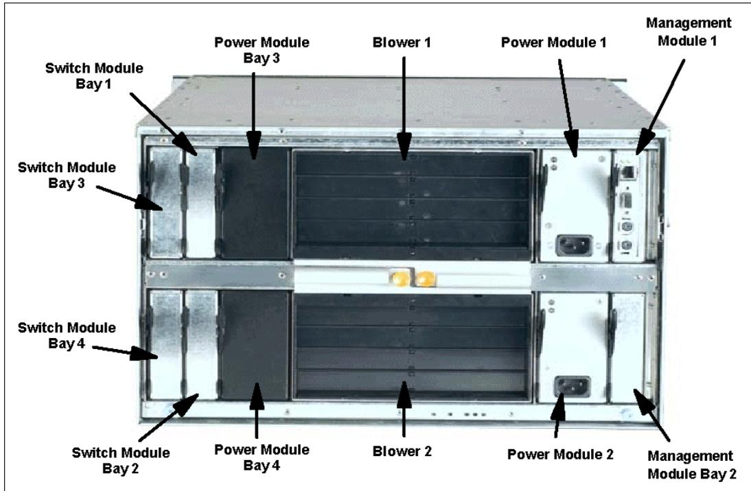
Figure 1-3 Rear view of BladeCenter chassis
