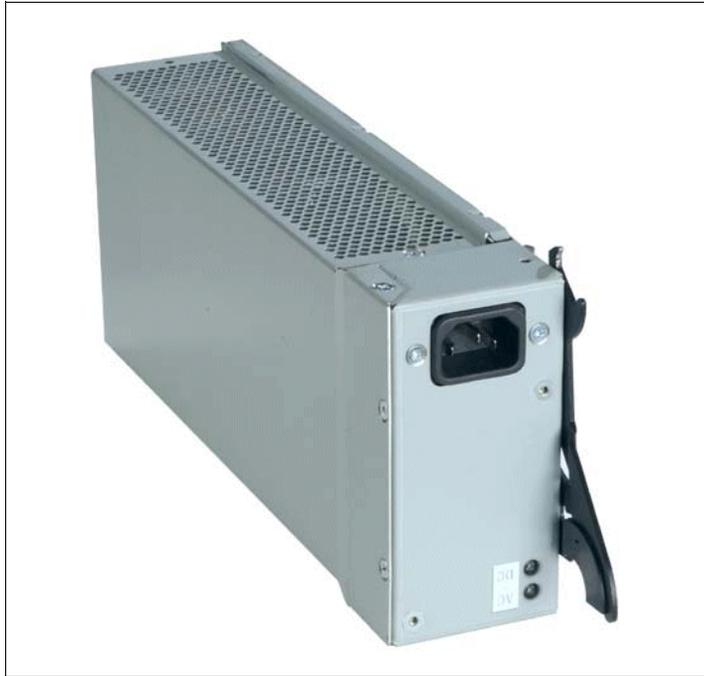
Figure 1-7 BladeCenter 1200W Power Supply Module
