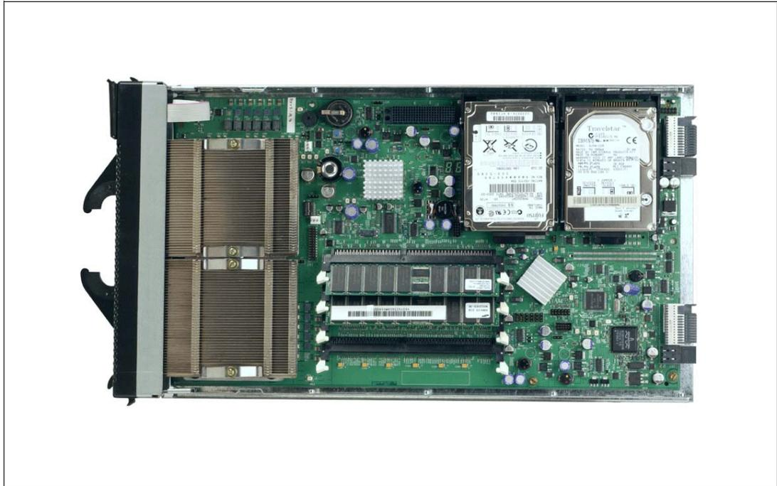
Figure 1-4 BladeCenter HS20 with top cover removed
