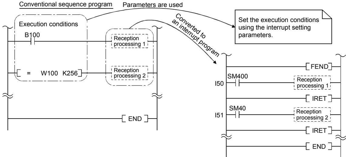
Interrupts generated by the link devices (LB/LW/LX) can be used for the normal cyclic transmission and direct access destinations.
