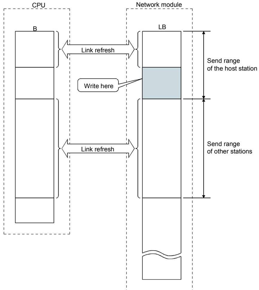
2) If an address within the link refresh range is designated, the data is written when the instruction is executed. However, the link device of the network module is overwritten with the link device data of the CPU by the link refresh.
