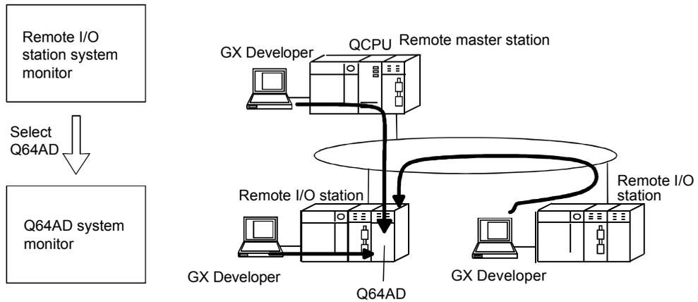
(b) If the GX Developer is connected to a remote I/O station, it will not affect the system operation so that the user program network function can be tested online.
