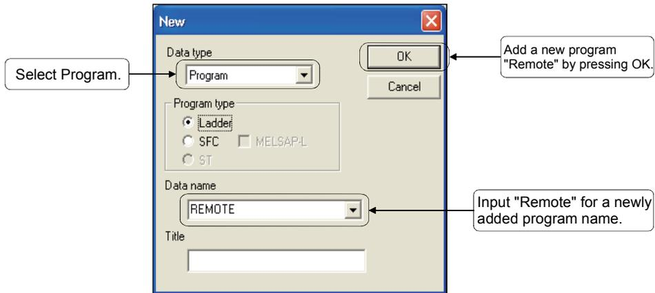
PLC 5 is operated by two programs: one for the PLC to PLC network (10NS5) and the other for the remote I/O network (20MR, 10R1).
