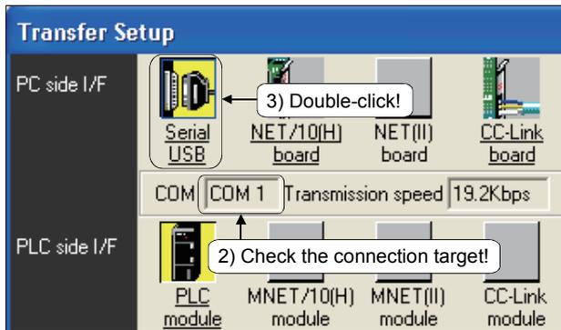
2) Check if the setting of the interfaces connected by the peripheral device and the CPU module matches.
