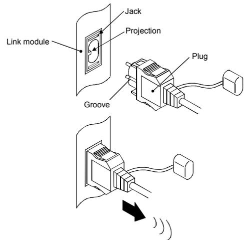
(3) Removing the optical fiber cable
