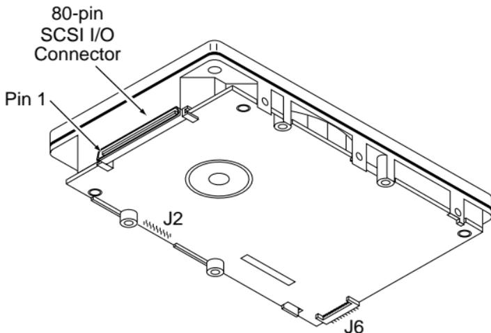
**Figure 14. 80-pin I/O connection to drive**
