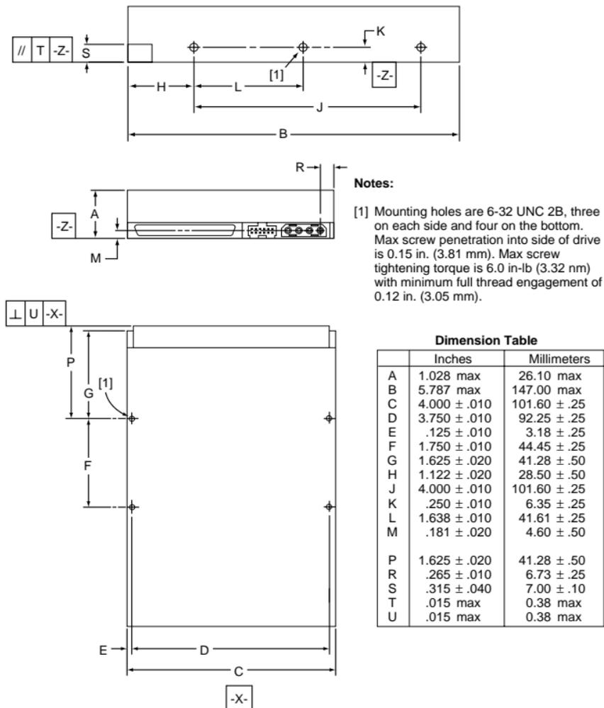
**Figure 10. Mounting configuration dimensions**
