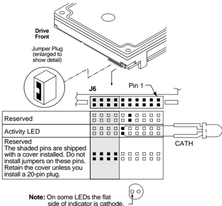
**Figure 6. Drive Active LED indicator connections**
