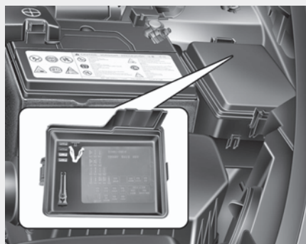
Engine compartment fuse panel
