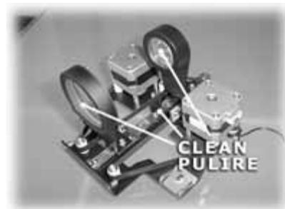
Once the frame with the Zoom/Focus mechanic unit has been removed, it is possible to clean the parts which are usually difficult to reach. Reassemble the Zoom/Focus unit carefully, being sure in particular that the blade with prism and frost is positioned between the two lenses of the Zoom/Focus unit. Remember then to connect again the 2 motors and the fan to their connectors.
