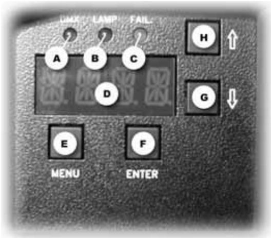
On the front panel of **MP700 Zoom** you'll find a section for the additional functions and for setting the projector.
