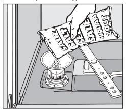
■ Place the funnel provided over the salt reservoir and carefully fill with salt until the reservoir is full. The salt reservoir holds approx. 2 kg of salt depending on the brand used.
