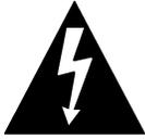
The lightning flash and arrowhead within the triangle is a warning sign indicating the presence of dangerous voltage.
