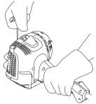
**CAUTION!** Do not pull the starter cord all the way out and do not let go of the starter handle when the cord is fully extended. This can damage the machine.
