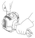
Once engine is started leave the choke lever in Half choke position for 20 seconds. Then move the choke lever to RUN position.
