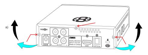
Unscrew the 3 securing screws. Hold the rear cover at its base as indicated by the blue arrows and twist outwards slightly and then lift the cover up.
