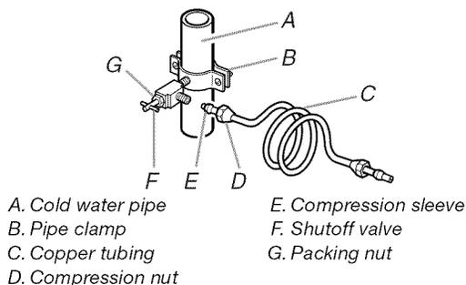
6. Fasten the shutoff valve to the cold water pipe with the pipe clamp. Be sure the outlet end is solidly in the 1/4" (6.35 mm) drilled hole in the water pipe and that the washer is under the pipe clamp. Tighten the packing nut. Tighten the pipe clamp screws slowly and evenly so the washer makes a watertight seal. Do not overtighten or you may crush the copper tubing.
