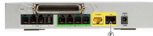
**STEP 6** Connect the included power adapter to the power port (G). Insert the power adapter into an electrical outlet. The power LEDs on the front panel are lit.
