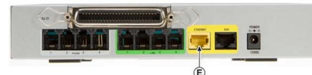
**STEP 5** Connect an one end of an Ethernet network cable to the AUX port (F). Connect the other end of the cable to the Ethernet port of your PC.
