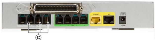
**STEP 3** For access to the PSTN (Public Switched Telephone Network), connect RJ-11 cables from the Line 1 to Line 4 FXO ports (D) to the RJ-11 wall outlet for the telephone service.
