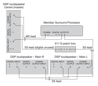
If your system includes more than two Meridian DSP loudspeakers you will need a 511 S-patch box (available separately) to link together the S5 leads from each speaker, as shown above. **Note:** This does not apply to the 861, which includes a built-in patch box.
