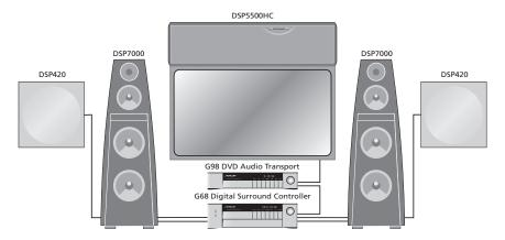
Up to seven Meridian DSP loudspeakers can be used in conjunction with a Meridian Surround Processor, such as the G68 Digital Surround Controller, to create a digital surround system with superb music and cinema sound.
