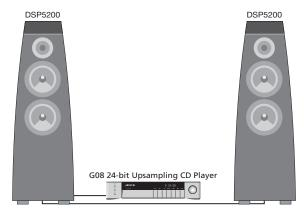
Meridian DSP loudspeakers include DSP volume and tone controls, and can be connected directly to up to two digital sources, such as the G08 24-bit Upsampling CD Player, to create an extremely compact high-quality music system.
