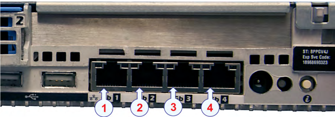
Figure 48 Ethernet connectors on the rear side of the TRC1–5 computers
