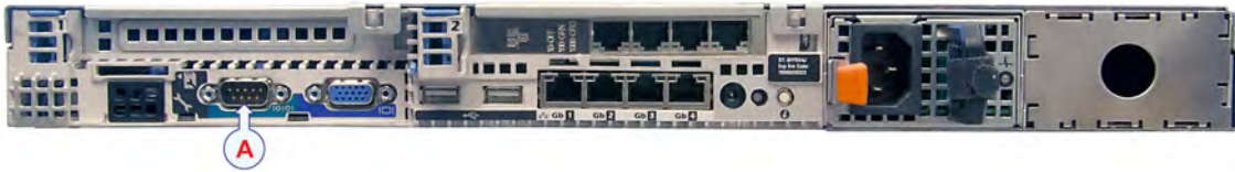
Figure 49 RS-232 connector on the rear side of the TRC0 Beamforming computer
