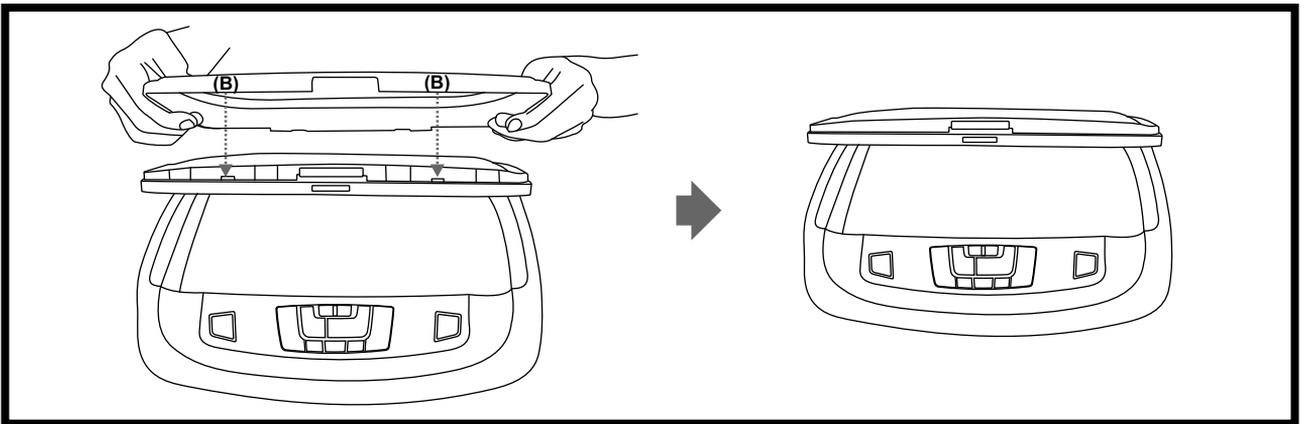
Open the screen and hook the two tabs "B" on the bottom edge of the screen. Snap the opposite side over the hinge.
