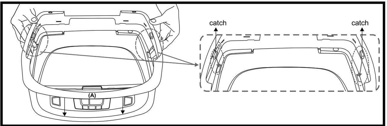
Begin by hooking area "A" (above) over the dome light and slide the cover over the pod. The cover will snap in place.
