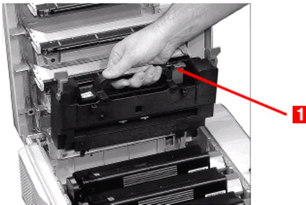
7. Push the two blue retaining levers (1) toward the rear of the printer to lock the fuser in place.
