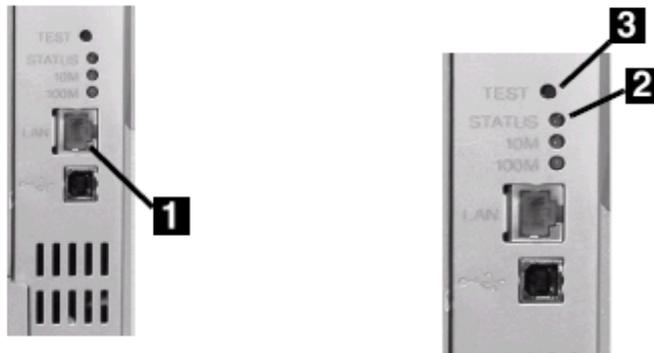
3. Turn the Printer ON and wait for the status light (2) to stop blinking.
