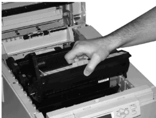
9. Remove the orange drum seal.
