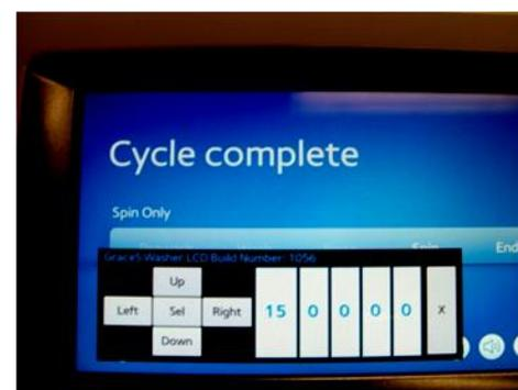
The cycle is now completed, but due to a spin issue, the unit never went over 500 RPMs, leaving the clothes wet.
