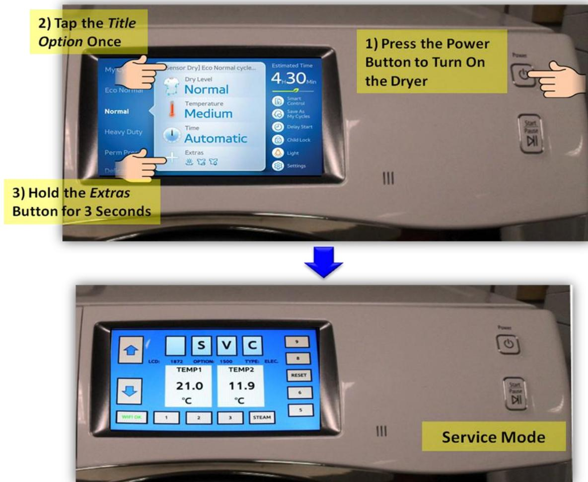
1. Press the Power Button to turn on the dryer.
