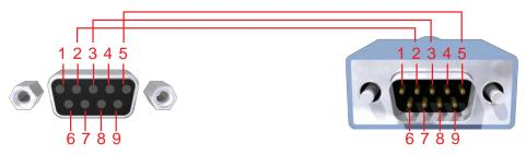
Only Pins 2 (RX), 3 (TX), and 5 (Ground) are needed to operate RS-232 Interface
