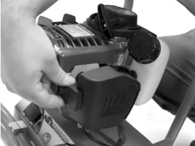
Step 1 – Remove carburetor cover by pressing clips.
