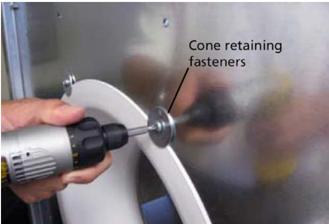
Figure 12: Loosen cone retaining fasteners
