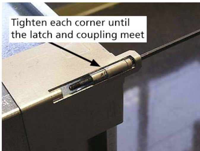
Figure F8: Tighten until latch and coupling meet
