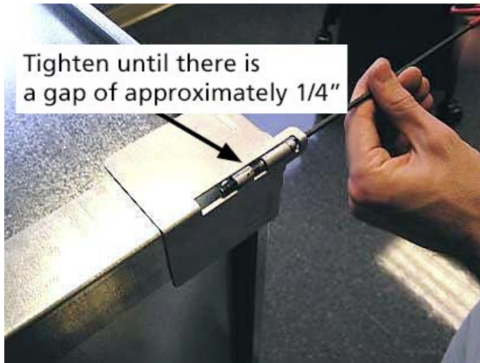
Figure F7: Tighten cap screw to ¼" of the coupling
