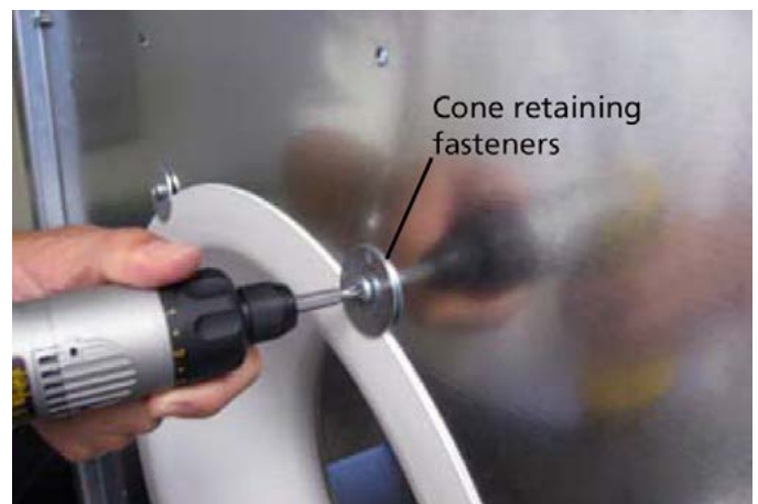
Figure 16: Tighten cone retaining fasteners
