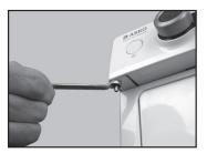
9. Slacken off the screws for the lower hinge on the corresponding side of the machine. This must be done to hang the door.
