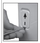
6. Carefully remove the catch and plastic plug on the door (according to the method above) and switch location.
