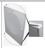
Method for removing plastic plugs, lock and catch located on the machine and the door: Carefully push the plug, catch or lock upwards with a flat screwdriver. as the picture shows.
