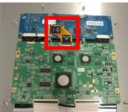
The LVDS cable pictured left is a directional cable, which means it will only function one way. To prevent the cables from being inserted incorrectly, we have clearly labeled each end.
