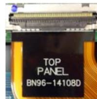
**Problem** – The UN55C9000, because of its unique design, offers some equally unique challenges when it comes to service. As you can see in the picture to the left, the LVDS cable is rather short, which limits its flexibility and makes inserting it into the FRC/TCon board and the docking board one of those challenges.
