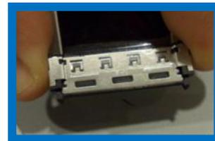
**Problem** – Due to the length and delicacy of the LVDS cable, it can sometimes be difficult to insert the cable after a main board assembly has been replaced.
