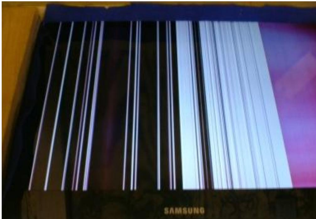
**Cure:** In this model, the T-CON has two output ICs that control the panel. Replace the T-CON. Before replacing the T-CON, reseal the LVDS cable.
