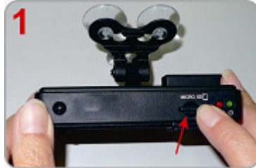
Force reduction SD card, SD card pop up lightly.
