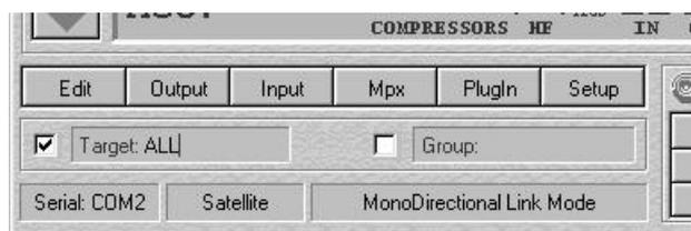
**Each processor 'responds' to the commands sent remotely (via the serial port 2) ONLY IF the Target Name and/or Group Name coincide, or if the password ALL is present.**
