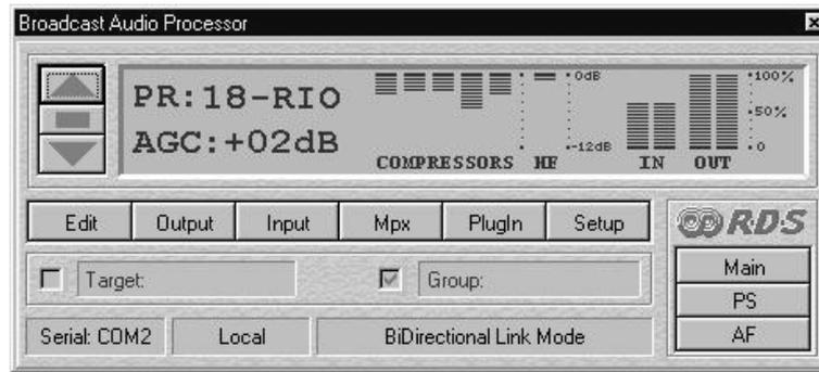
It has a window with a yellow-green background quite similar to that of the front panel of the processor. The serial port of the computer being used and the current connection mode are indicated at the bottom of the window.
