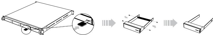
**Step-2:** Place the hard drive into the tray, and fasten the screws in the corresponding locations. Place the tray with the mounted hard drive back into the enclosure. (If the screws are not properly fastened, the hard drive may be pushed towards the back of the unit and the tray handle will not open properly.)
