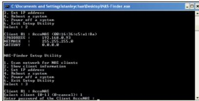
**NOTE:** DHCP is pre-defined for LAN port-1. DHCP is used to quickly assign a local IP to the NAS unit. Changing the IP address to a static IP address is strongly recommended for daily operations.
