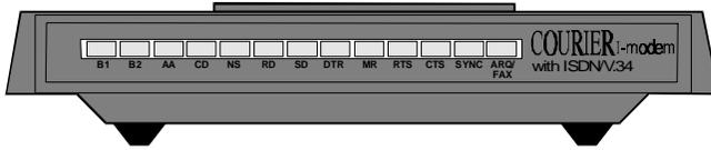
**Figure 5.1 Front panel of the I-modem**
