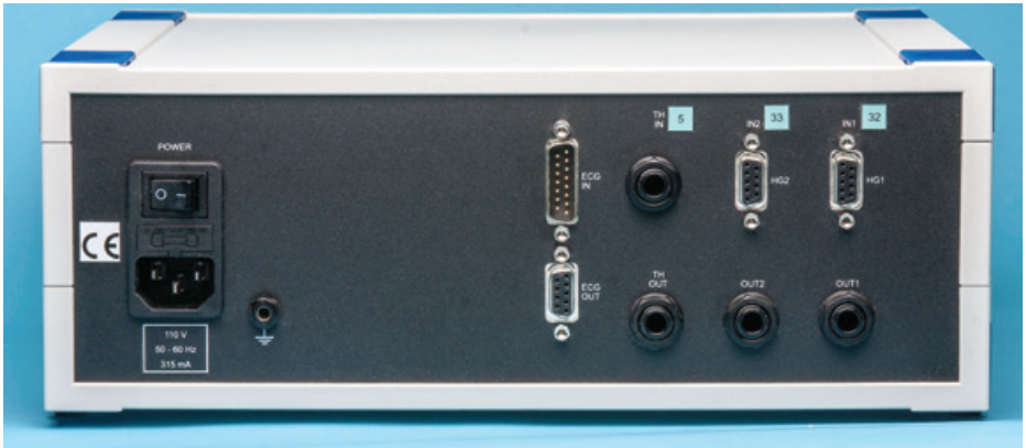
Fig. 3—The back panel has the input and output sockets, along with the main power switch.
