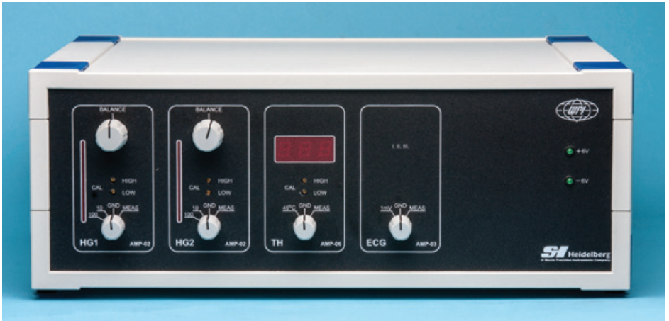
Fig. 1—The Biological Signals Amplifier has four modules.
