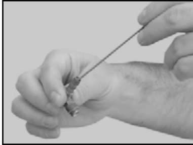
(E) Clean the Blade Guard Intake Fitting
