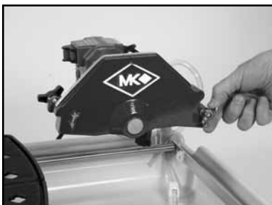
(A) Loosen the Blade Guard Retaining Wingnut
