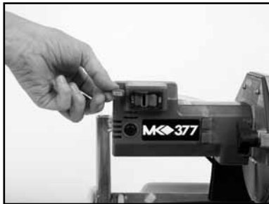
(B) Lockout the Saw by removing the Lockout Pin
