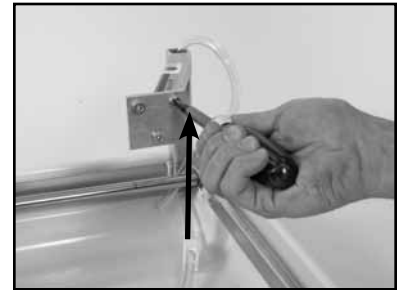
(C) Locate and remove the three Cutting Head Retaining Screws using a Phillips Screwdriver
