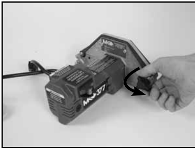
(A) Loosen the Blade Guard Retaining Knob
