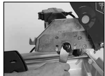
(C) Place the Shaft Wrench on the Motor Shaft (NOTE: the Outer and Inner Flanges and the Blade Nut are removed in the photo above) rotate blade shaft so shaft wrench is engaged.
