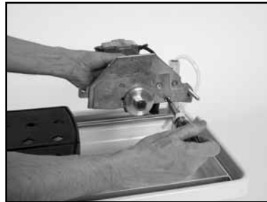
(E) Install the three Cutting Head Retaining Screws using a Phillips Screwdriver
