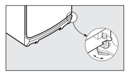
To align the appliance adjust the feet using the spanner supplied.
