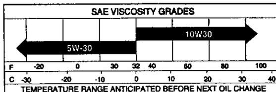
Change the oil after every 50 hours of operation or at least once a year if the tractor is not used for 50 hours in one year.
