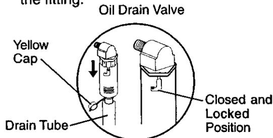
3. Unlock drain valve by pushing upward slightly and turning counterclockwise.
