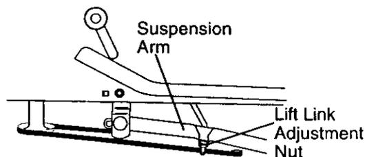
Check adjustment on right side of tractor. Position any blade so the tip is pointing straight forward. Measure distance "B" at front and rear tip of blade
