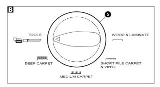
Before using the cleaner, the floor nozzle height 5 must be set to the correct height.
