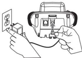
**D** Place the handset in the base and charge continuously for 15 - 20 hours before using the phone.
