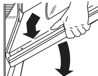
2. Hold oven door so that the top edge of each door slot is horizontal. Insert door hinge into the hinge slots.
