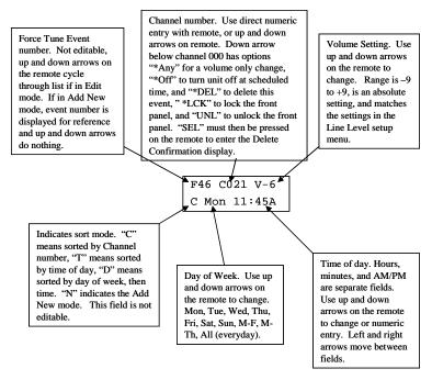
The left/right arrows on the remote move the cursor through the fields that can be changed. The settings for each of the fields are selected using the up/down keys on the remote.
