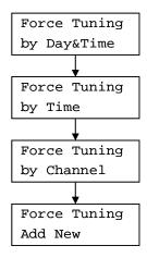
Forced Tuning is an advanced feature for the commercial market that allows programmed events to occur throughout the day or week in an unattended manner. These events can program the unit to turn on or off, lock and unlock the front buttons, change channel, and change volume. Up to 100 events may be programmed in the XM-100.
