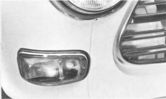
Unscrew the two screws by means of a Philips screwdriver and lift off the glass and the metal frame. The bulbs can now be removed by pushing in and twisting anti-clockwise.
