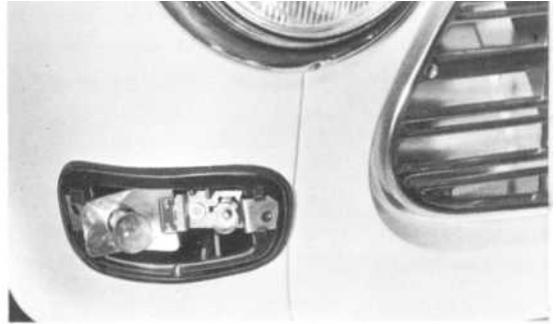
The larger one is the flasher and the smaller one the parking light. See that the glass seats properly on the gasket.
