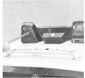
The number plate lighting is built into the handle on the luggage compartment lid with one bulb on each side of the emblem. The bulbs are accessible from the underside of the emblem.
