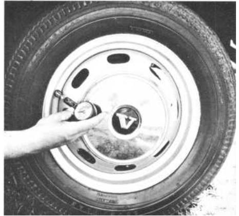
Excessively low air pressure is one of the most usual reasons for wear. If pressure is too low, the outer edges of the tread take the whole loading and wear down very quickly. Insufficiently inflated tyres also result in difficult steering and high fuel consumption.
