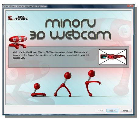
First place Minoru on the desk or on the top of your monitor at a distance of about 3 feet (1 metre) from your face. At this stage you should not wear the 3D glasses.
