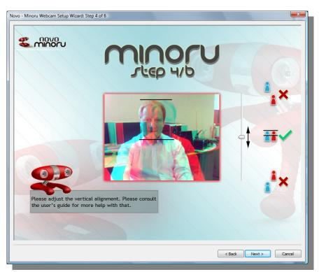
Vertical alignment...At this point you should still not wear the 3D glasses. Look at Minoru and you should see two images of your face on the screen, a blue image and a red image. Adjust the vertical slider so that the red and blue images of your face are at exactly the same height on the screen. Sometimes it is easiest to look at the top or bottom of your head or at your eyes in order to align the two images.
