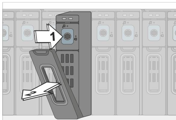
Figure 5-2: Pulling out the lever
