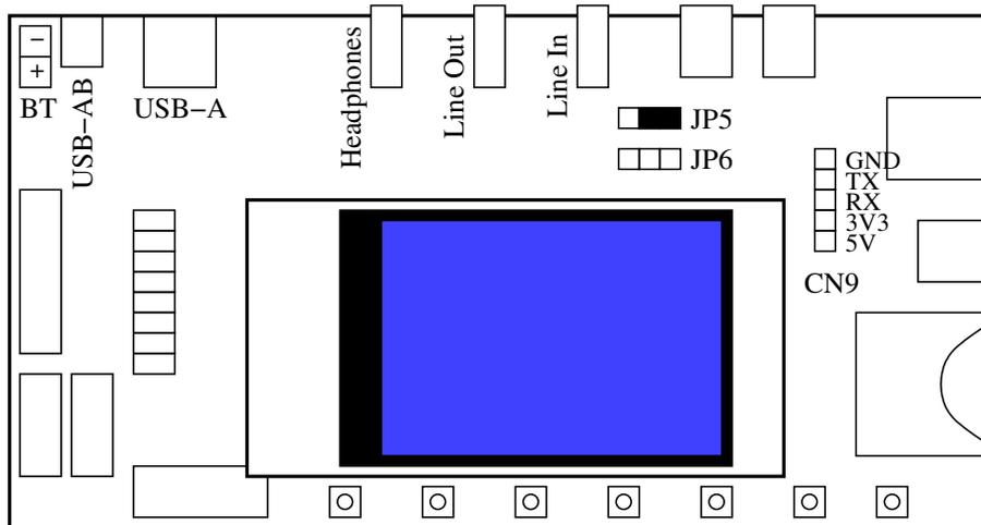
Figure 1: VS1005 Developer Board.
