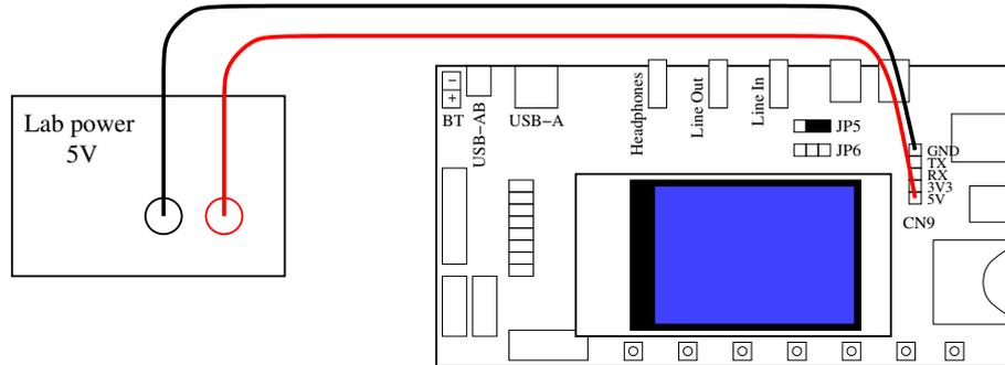
Figure 2: VS1005 Developer Board with lab power.
