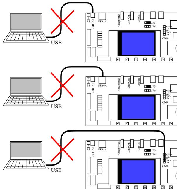
Figure 4: For proper measurement results, do *not* power the VS1005 Developer Board from a PC computer port. Use a stabilized laboratory power or a battery as shown in Figures 2 and 3.
