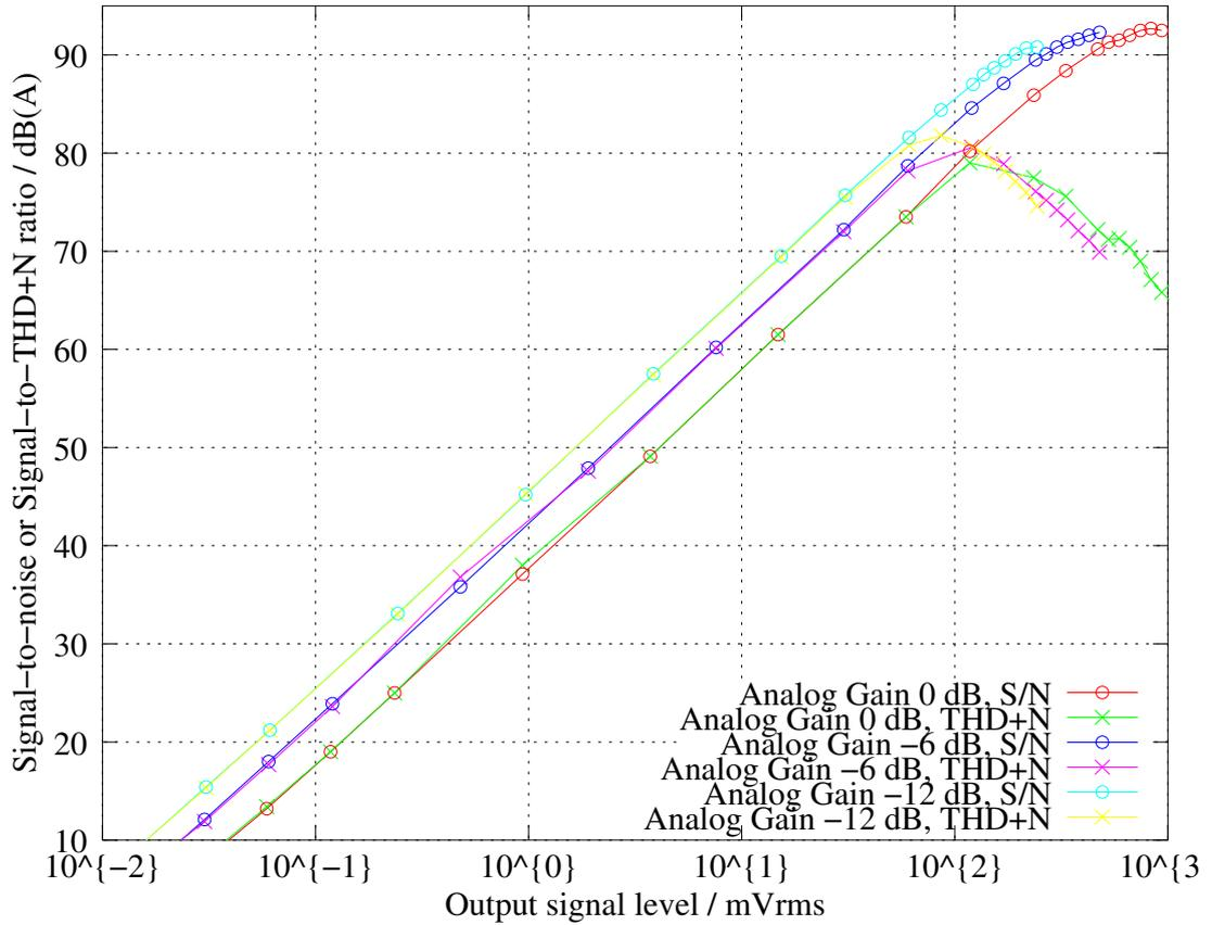
Figure 14: VS1005 DevBoard output signal to noise and THD+N ratios at different output signal levels.
