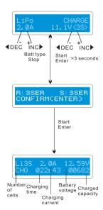
The left side of the first line shows the type of battery you select at the users setting. The value on the left side of second line sets a charge current and the value on the right side of second line sets the voltage of the battery pack.
