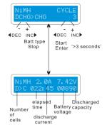
To stop the process,press Batt.Type/Stop key once. You can change the discharge or charge current by pressing Start/Enter key once during the process. The audible sound indicates you the end of process.
