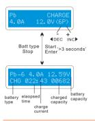
Set up the charge current on the left and the nominal voltage of the battery on the right. The charge current ranges from 0.1 to 10.0A and the voltage should be matched with the battery being charged.
